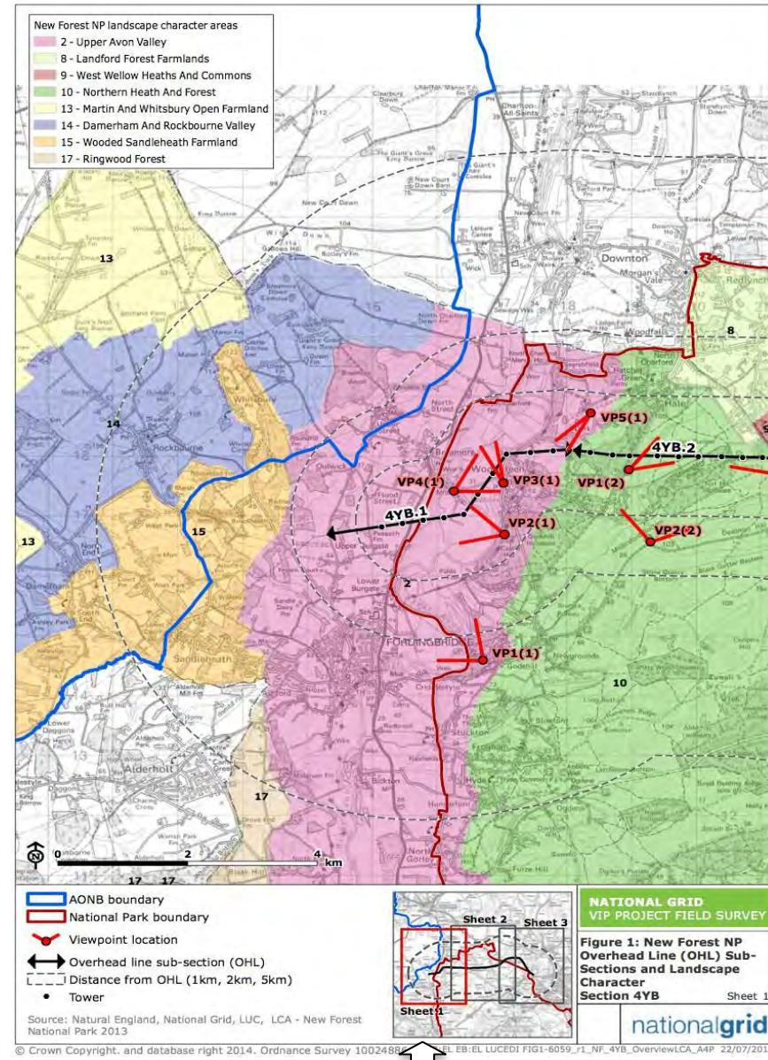
Figure 1 shows the line subsection and towers/pylons overlaid on landscape character types/areas and with viewpoints and direction of view. VP2 (1) means viewpoint 2 for subsection 1
